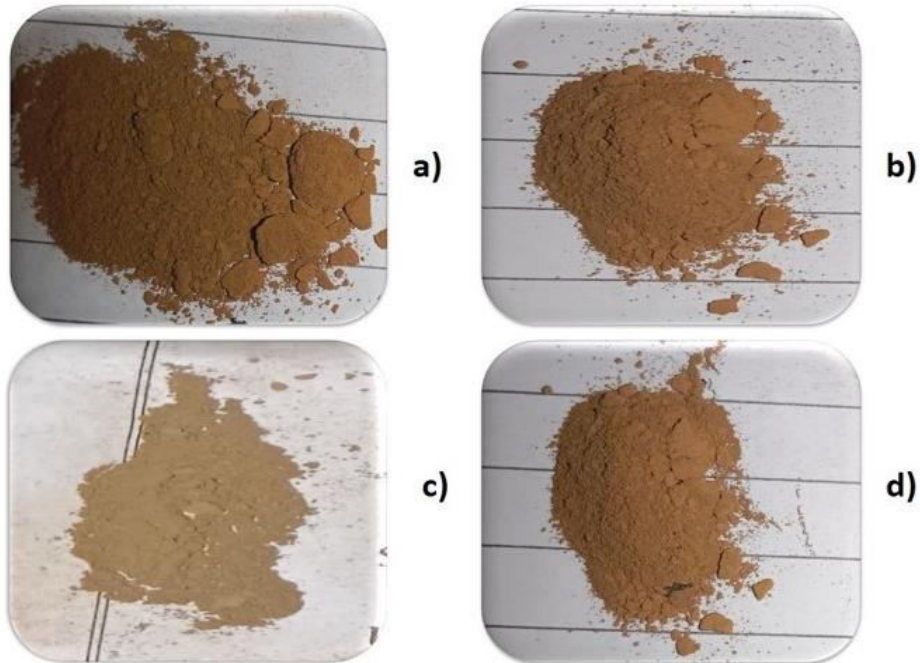
Fig. 2 (a), (b), (c), (d) shows the synthesized powders of \text{Bi}_{0.95}\text{Zn}_{0.05}\text{Fe}_{0.95}\text{Ni}_{0.05}\text{O}_3 , \text{Bi}_{0.9}\text{Zn}_{0.1}\text{Fe}_{0.9}\text{Ni}_{0.1}\text{O}_3 , \text{Bi}_{0.85}\text{Zn}_{0.15}\text{Fe}_{0.85}\text{Ni}_{0.15}\text{O}_3 and \text{Bi}_{0.8}\text{Zn}_{0.2}\text{Fe}_{0.8}\text{Ni}_{0.2}\text{O}_3 ceramic samples.
